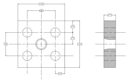
3. Using subprogram - Create a part program for mirroring and produce component in the Machine.
