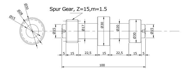
Exercise No:5- Spur Gear milling (Differential Indexing)
