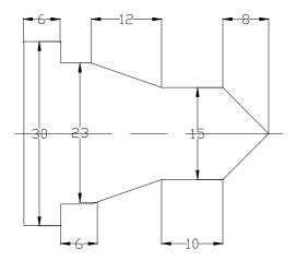
3. Create a part program for circular interpolation and simulate in the software - Using Circular interpolation.
