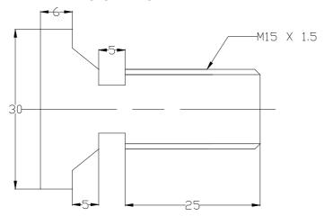
6. Create a part program for internal drills, boring and simulate in the software.
