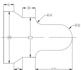
4. Create a part program for multiple turning operations and simulate in the software - Using Stock removal cycle.
