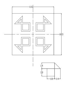
4. Create a part program for rectangular and circular pocketing and simulate in the software - Using canned cycle.
