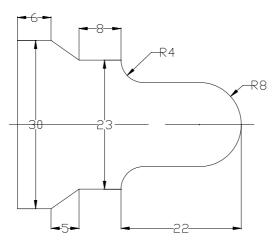
3. Using Stock removal cycle – Create a part program for multiple turning operations and produce component in the Machine.
