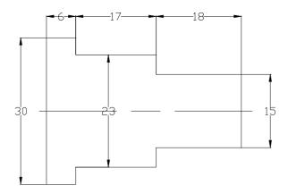
2. Create a part program for taper turning and simulate in the software - Using Box turning cycle.
